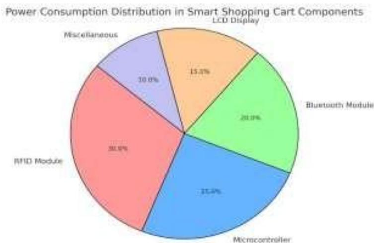
Figure 3: Component-wise Power Consumption
