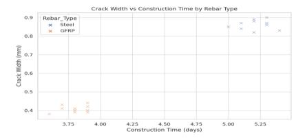
Construction time vs. crack width scatter plots depict the direct correlation between construction duration and crack width. GFRP reinforced slabs show shorter construction times and significantly greater resistance to cracking when compared to steel reinforced slabs.
