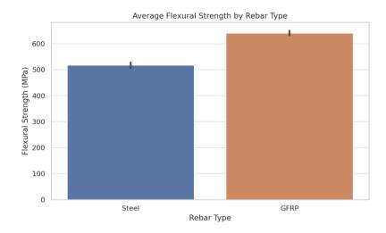
This vertical bar graph depicts comparison of flexural strength of GFRP and steel reinforced slabs (MPa). GFRP slabs not only outperform steel slabs, but also have a more consistent performance which indicates lower variability.
