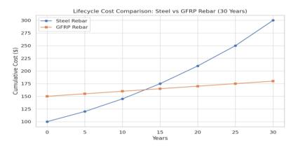
**Description:** A line chart illustrating the long-term cost projection for maintenance and replacement of steel rebar surpassing GFRP costs over a period of thirty years.
