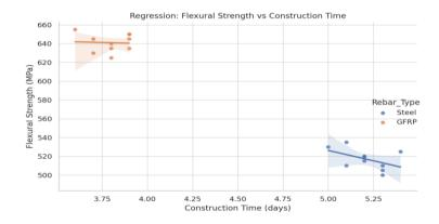
Construction time dependent flexural strength visualization is represented in this regression plot along with the trend lines segmented by rebar type. Supplementary data shows that with GFRP, not only faster construction is achieved but also greater strength is realized.
