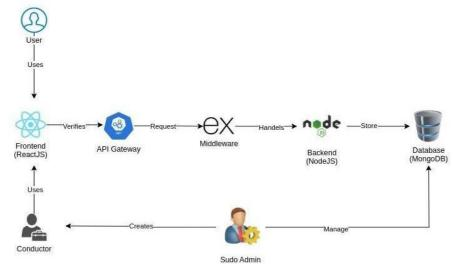
A number of interconnected parts make up the suggested system architecture for India's digital ticketing system for public bus transit, enabling a smooth and effective ticketing procedure. Let's examine each part and how it works:
